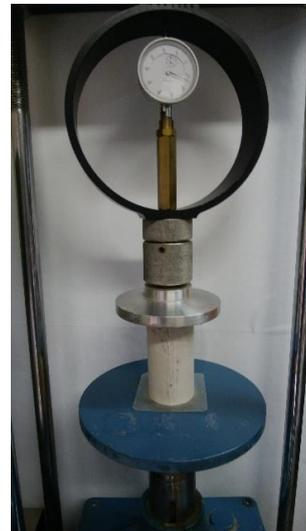
Fig.3 Uniaxial compression test
